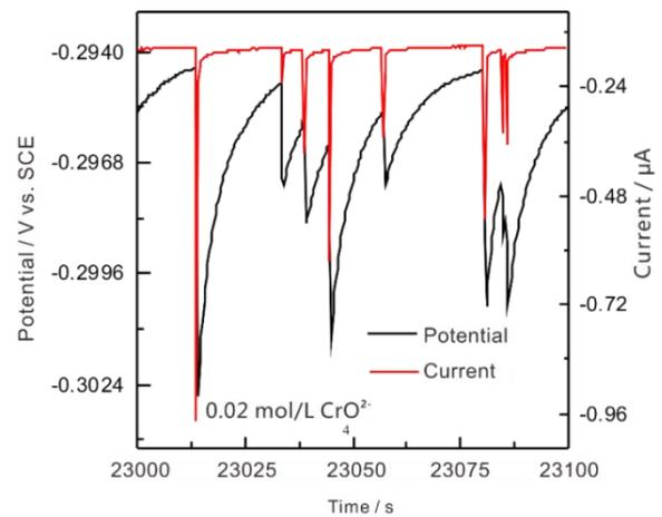
EN of low-carbon steel in 0.05mol/LCl<sup>-</sup>+0.1mol/LNaHCO<sub>3</sub>
