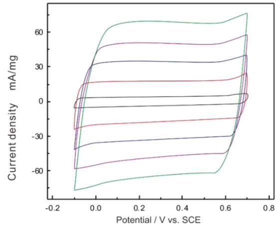
CV curve of PPy supercapacitor in 0.5 mol/L H<sub>2</sub>SO<sub>4</sub> solution
